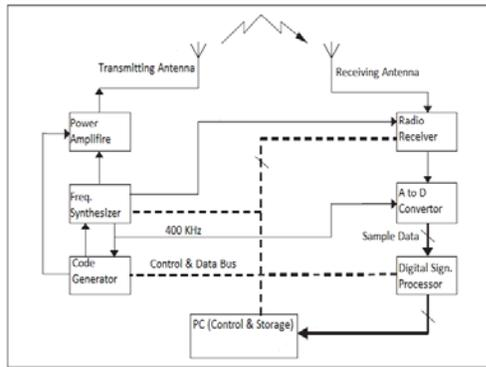
**Fig. 2: Simplified Functional diagram of a digital Ionosonde.**
